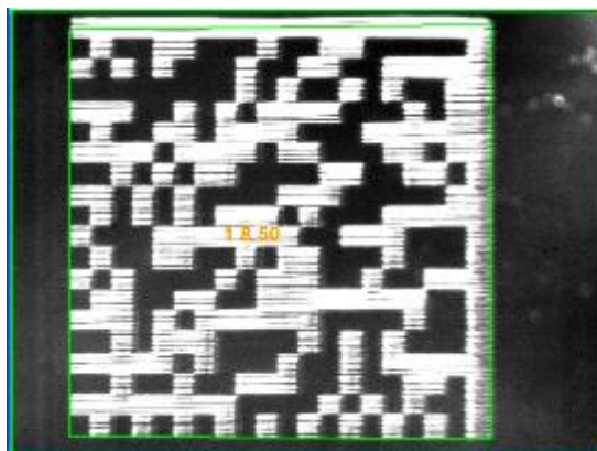
Engraving of a 1x1mm code in a pharmaceutical vial
