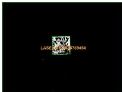
0.5x0.5mm surface engraving on black tinted glass
