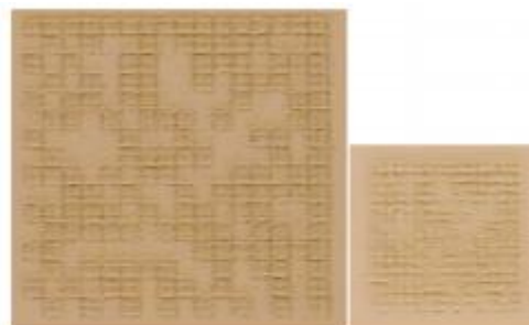
200µm and 100µm datamatrix with cross-hatch engravings
