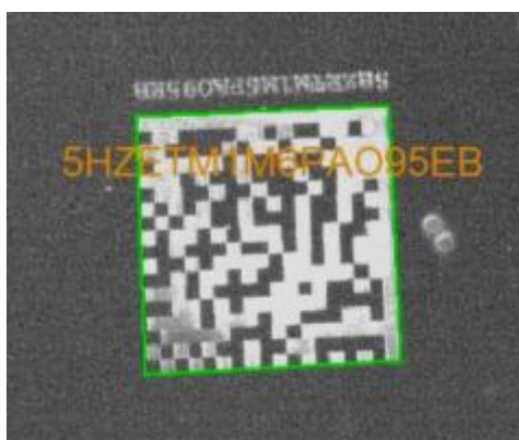
Reading of a 500µmx500µm datamatrix
