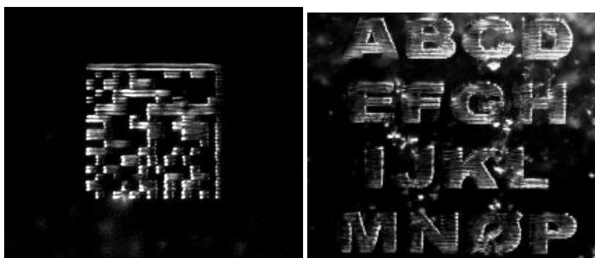
0.3mm code and 1mm text engraved at 0.1mm deep
