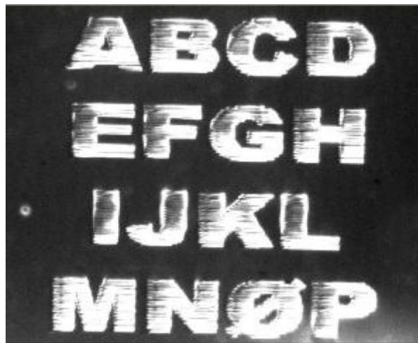
Text engraving (1x1mm) at 0.1mm deep
